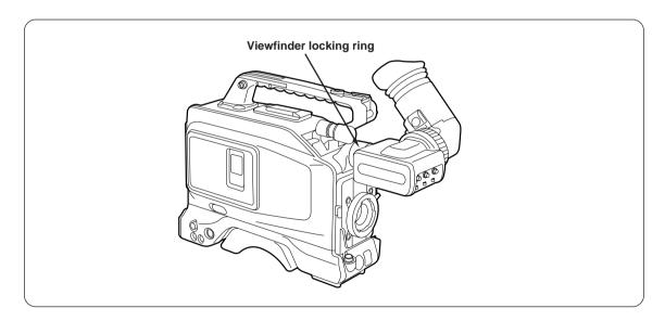
The viewfinder can be turned by 90 degrees by loosening the locking ring.
